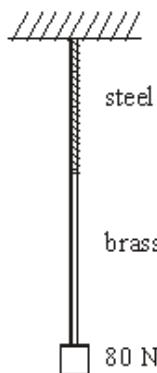
Each wire has a cross-sectional area of  $2.4 \times 10^{-6} \text{ m}^2$ .
